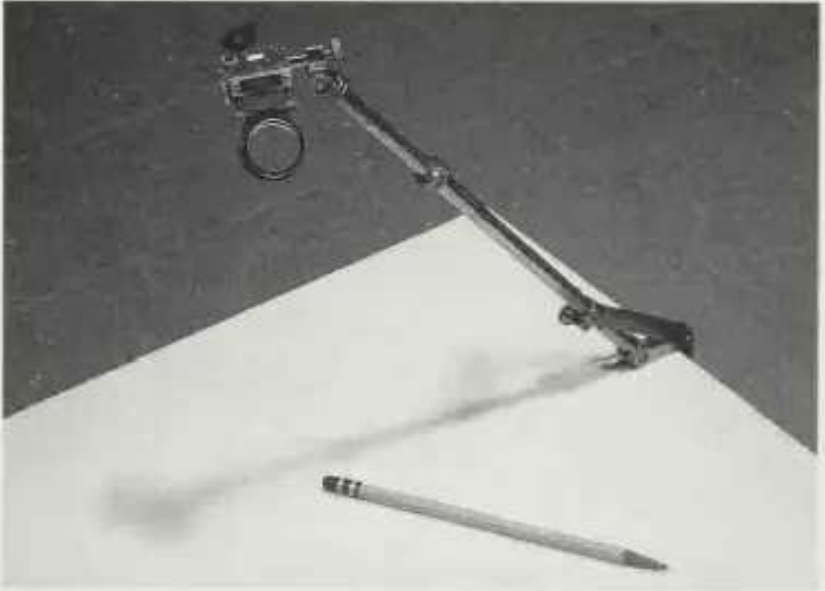
An early nineteenth-century camera lucida attached to a drawing table
